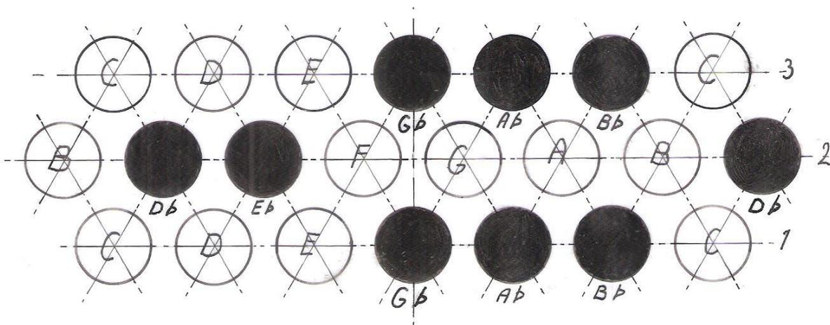
Figure 1 New chromatic keyboard for one octave with three rows of keys
