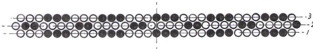
Figure 2 New chromatic keyboard for a 5-octaves keyboard
