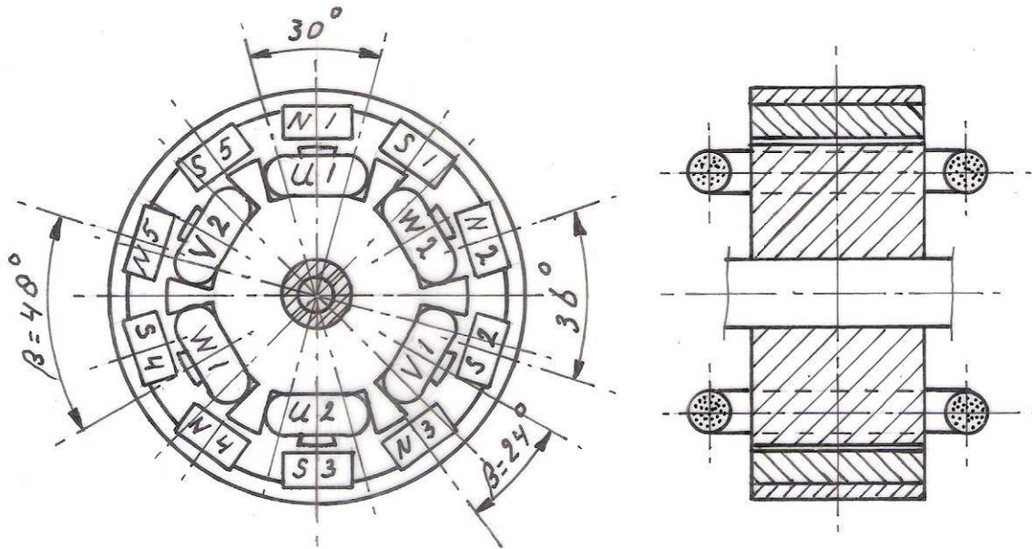
Figure 2 Armature and stator of a 10-pole, 3-phase hub dynamo
