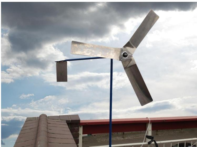
The VIRYA-1.04 using a NEXUS hub dynamo as generator
