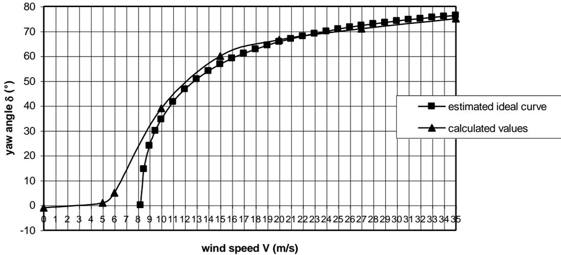
figure 13 The estimated ideal en the calculated  $\delta$ -V curve of the VIRYA-4.2 windmill
