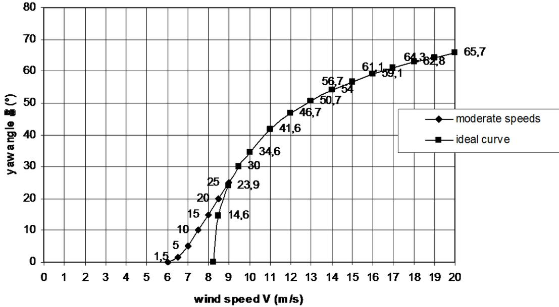
figure 5 Estimated  $\delta$ -V curve of the VIRYA-4.2 windmill
