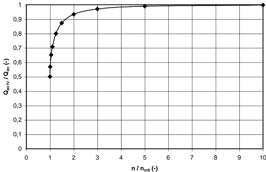
fig. 4 Values of  $Q_{av\ fv} / Q_{av}$  as a function of  $n / n_{crit}$
