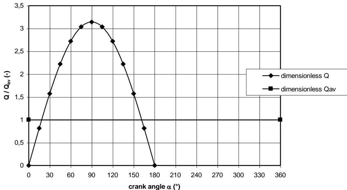
fig. 1 Dimensionless torque  $Q / Q_{av}$  and dimensionless average torque  $Q_{av} / Q_{av}$  as a function of the crank angle  $\alpha$
