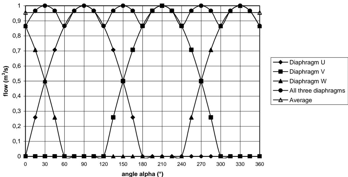
fig 1 fluctuation of the flow of each diaphragm q and of the total flow q<sub>tot</sub> for C = 1.
