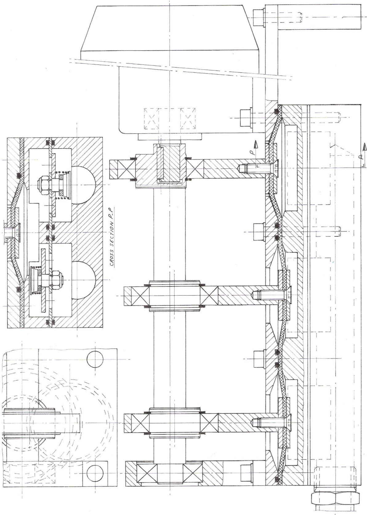
fig. 2 Diaphragm pump with three connecting rods
