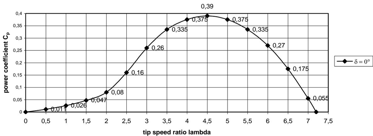
fig. 3 Estimated  $C_p$ - $\lambda$  curve for the VIRYA-1.66 rotor for the wind direction perpendicular to the rotor ( $\delta = 0^\circ$ )
