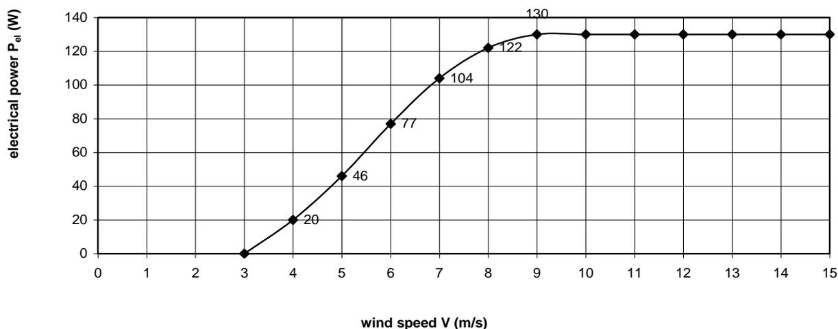
fig. 7 Estimated  $P_{el}-V$  curve of the VIRYA-1.66 windmill with  $V_{rated} = 9$  m/s for 12 V battery charging
