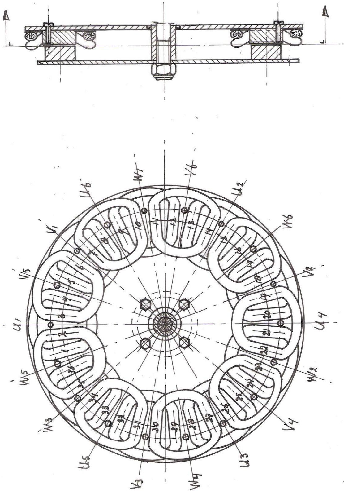
fig. 8 Alternative 2-layers, 3-phase winding for VIRYA-1.66 generator
