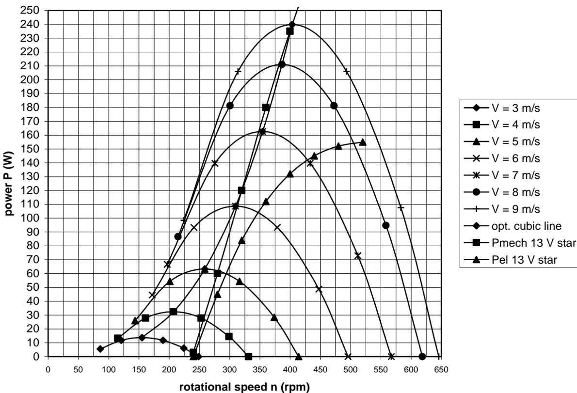
fig. 6 P-n curves of the VIRYA-1.66 rotor, optimum cubic line, estimated  $P_{mech-n}$  and  $P_{el-n}$  curves for 12 V battery charging for the chosen winding rectified in star
