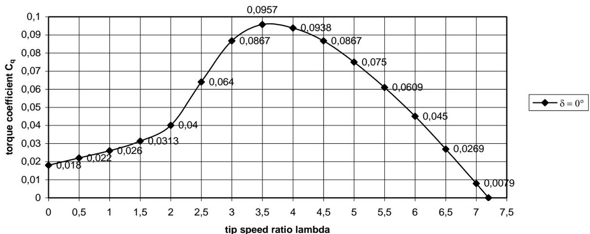
fig. 4 Estimated  $C_q$ - $\lambda$  curve for the VIRYA-1.66 rotor for the wind direction perpendicular to the rotor ( $\delta = 0^\circ$ )
