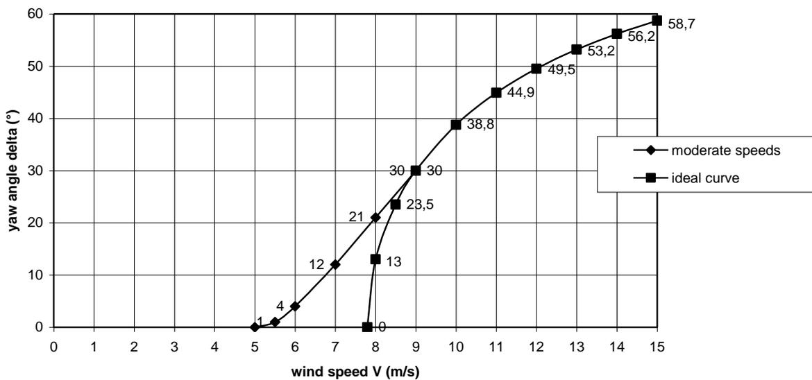
fig. 5 Estimated  $\delta\text{-V}$  curve VIRYA-1.66 for a 2 mm aluminium vane blade
