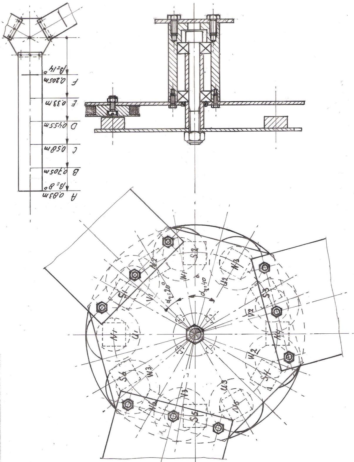
fig. 1 12-pole axial flux permanent magnet generator VIRYA-1.66
