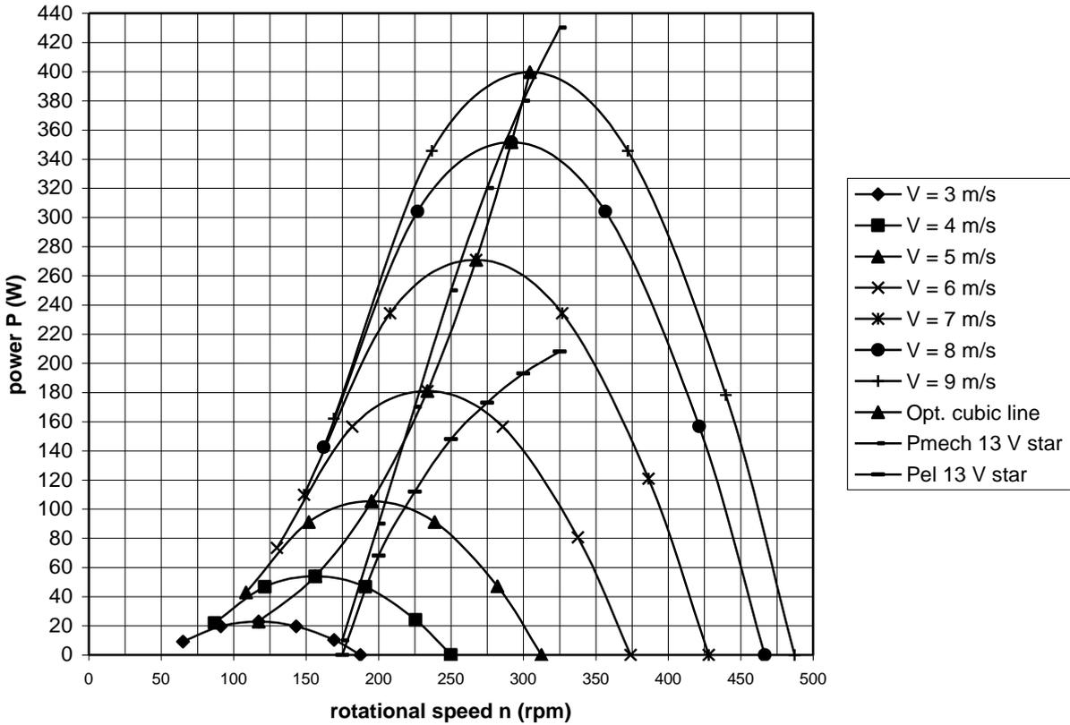
fig. 6 P-n curves of the VIRYA-2.2 rotor, optimum cubic line, estimated  $P_{mech-n}$  and  $P_{el-n}$  curves for 12 V battery charging for the chosen winding rectified in star
