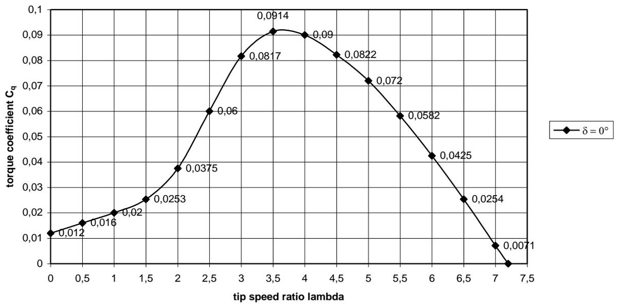
fig. 4 Estimated  $C_q$ - $\lambda$  curve for the VIRYA-2.2 rotor for the wind direction perpendicular to the rotor ( $\delta = 0^\circ$ )
