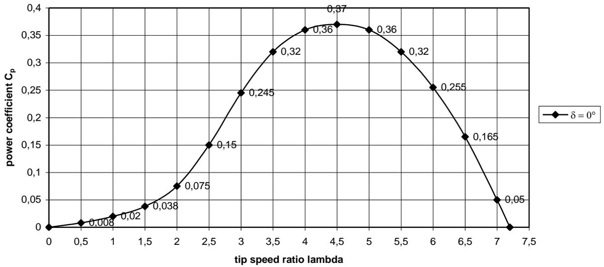
fig. 3 Estimated  $C_p$ - $\lambda$  curve for the VIRYA-2.2 rotor for the wind direction perpendicular to the rotor ( $\delta = 0^\circ$ )
