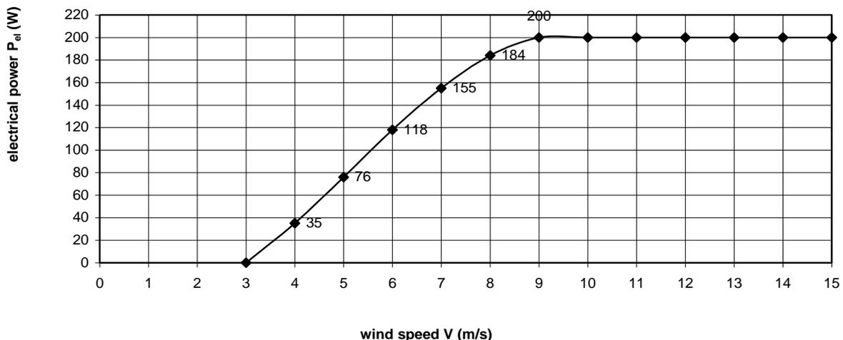
fig. 7 Estimated  $P_{el}-V$  curve of the VIRYA-2.2 windmill with  $V_{rated} = 9$  m/s for 12 V battery charging
