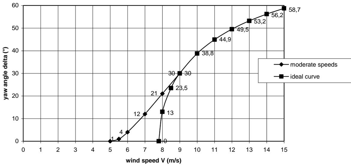
fig. 5 Estimated  $\delta\text{-V}$  curve VIRYA-2.2 for a 2 mm aluminium vane blade
