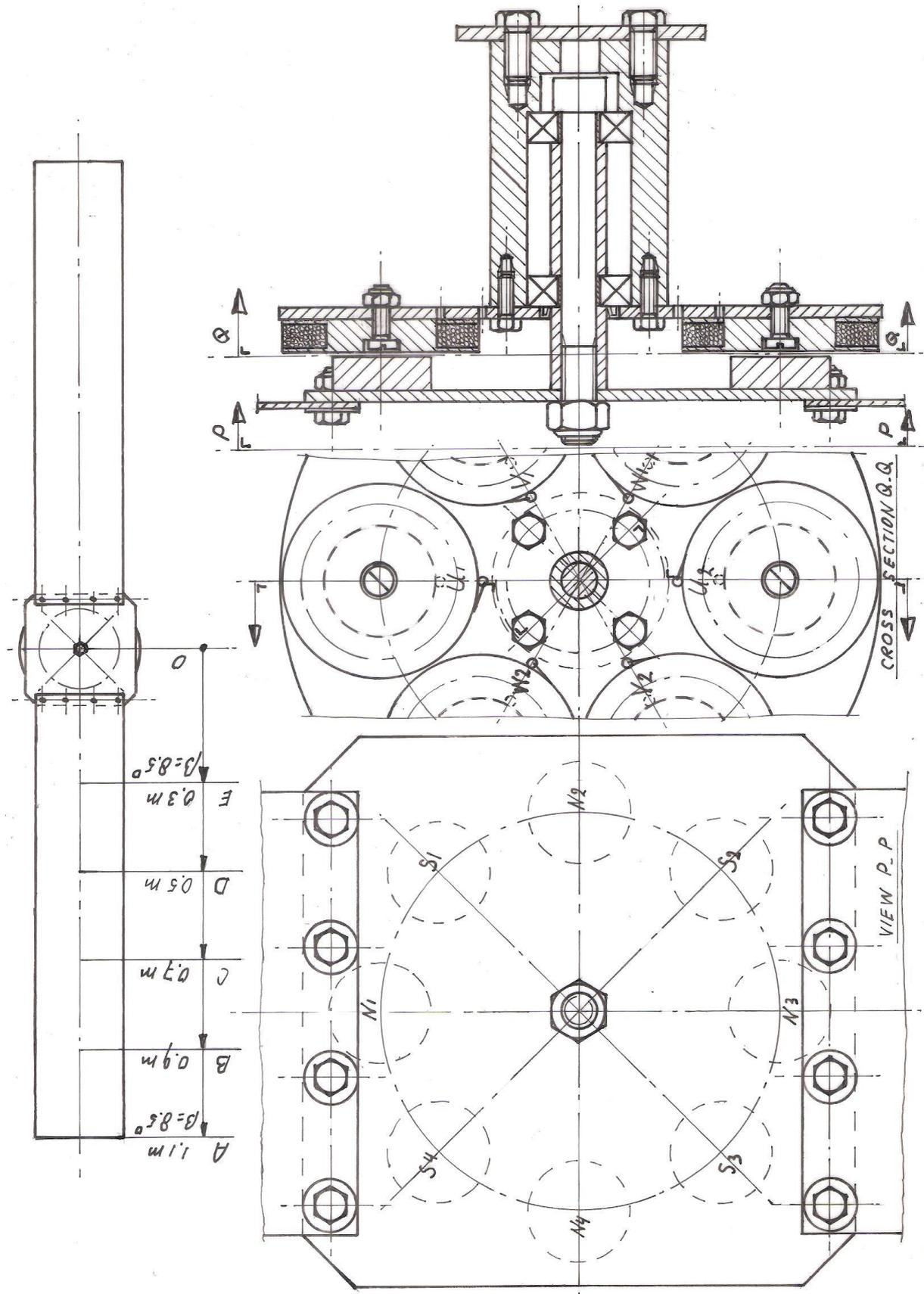
fig. 2 8-pole axial flux permanent magnet generator VIRYA-2.2
