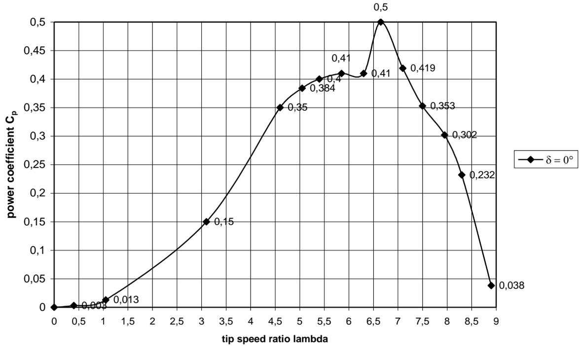
fig. 2 Measured  $C_p$ - $\lambda$  curve for a 2 mm stainless steel rotor for a tunnel wind speed of 11 m/s
