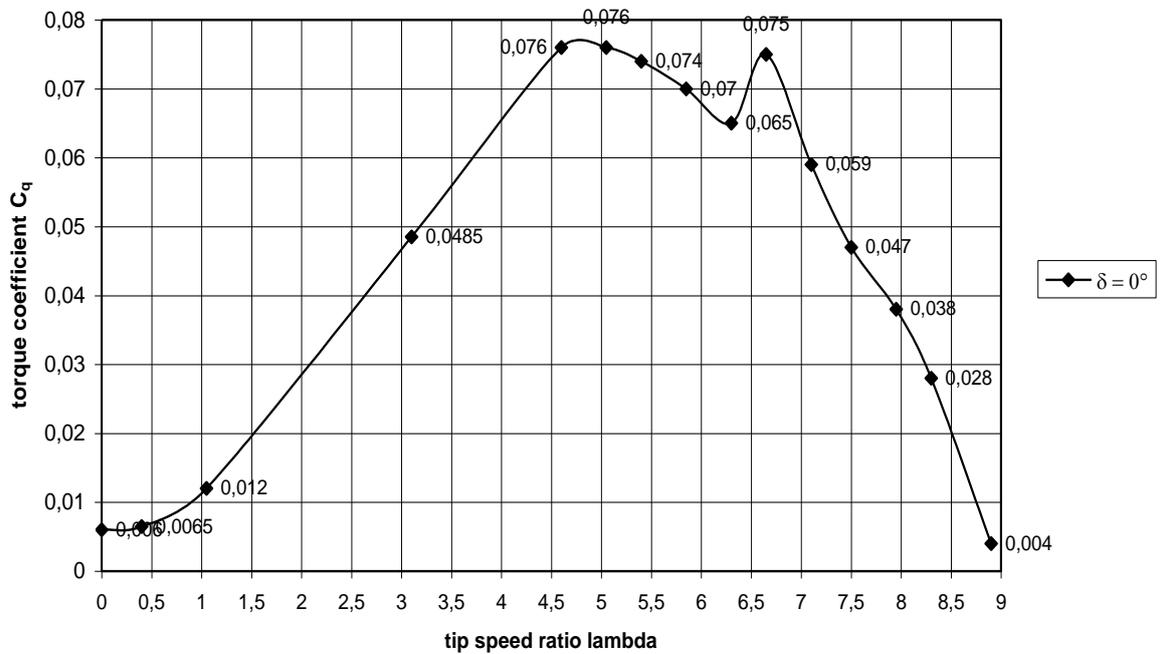
fig. 3 Measured  $C_q$ - $\lambda$  curve for a 2 mm stainless steel rotor for tunnel wind speed of 11 m/s
