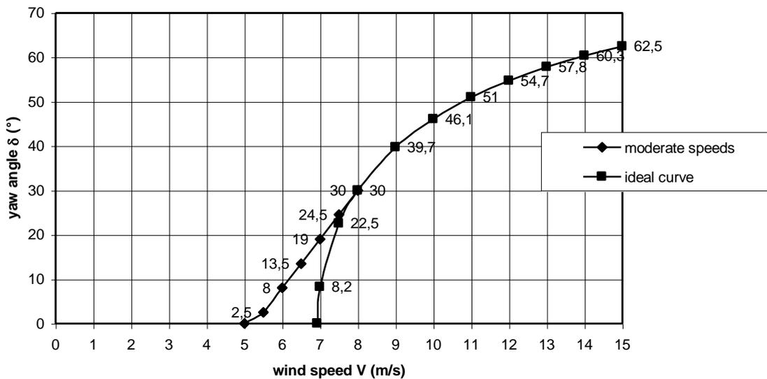
fig. 4 Estimated  $\delta\text{-V}$  curve VIRYA-3.4 safety system with  $V_{\text{rated}} = 8$  m/s
