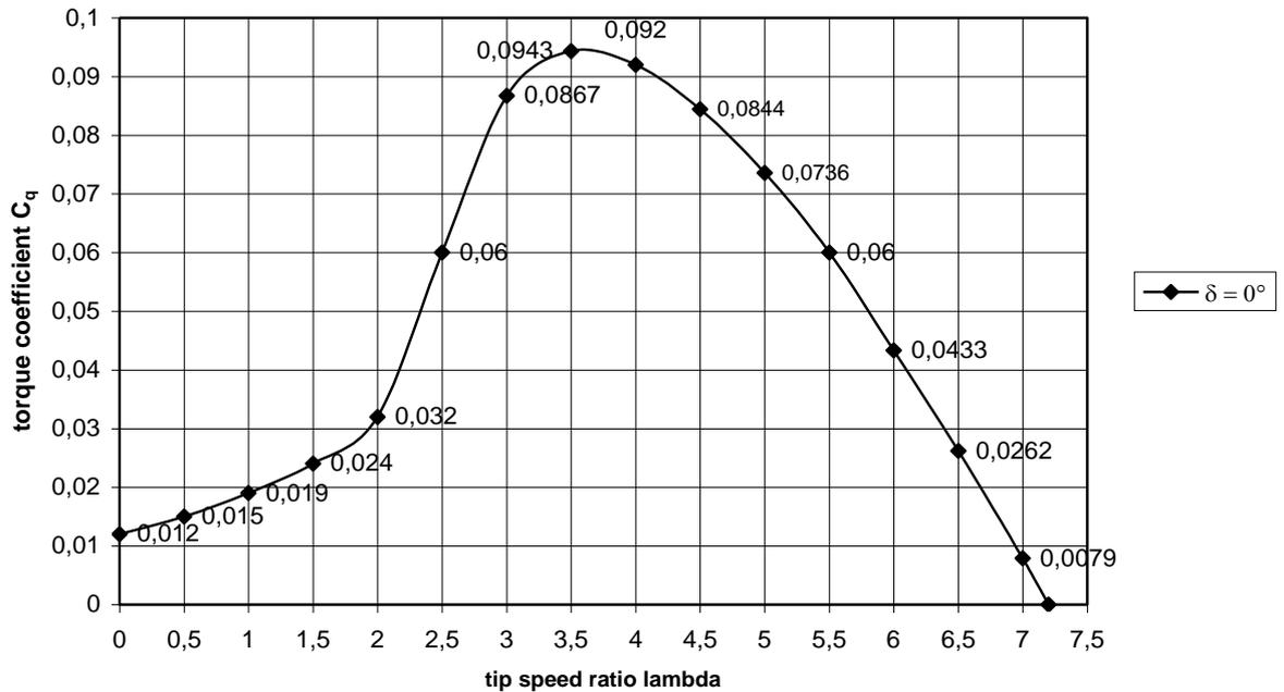
fig. 3 Estimated  $C_q$ - $\lambda$  curve for the VIRYA-3.4 rotor for the wind direction perpendicular to the rotor ( $\delta = 0^\circ$ )
