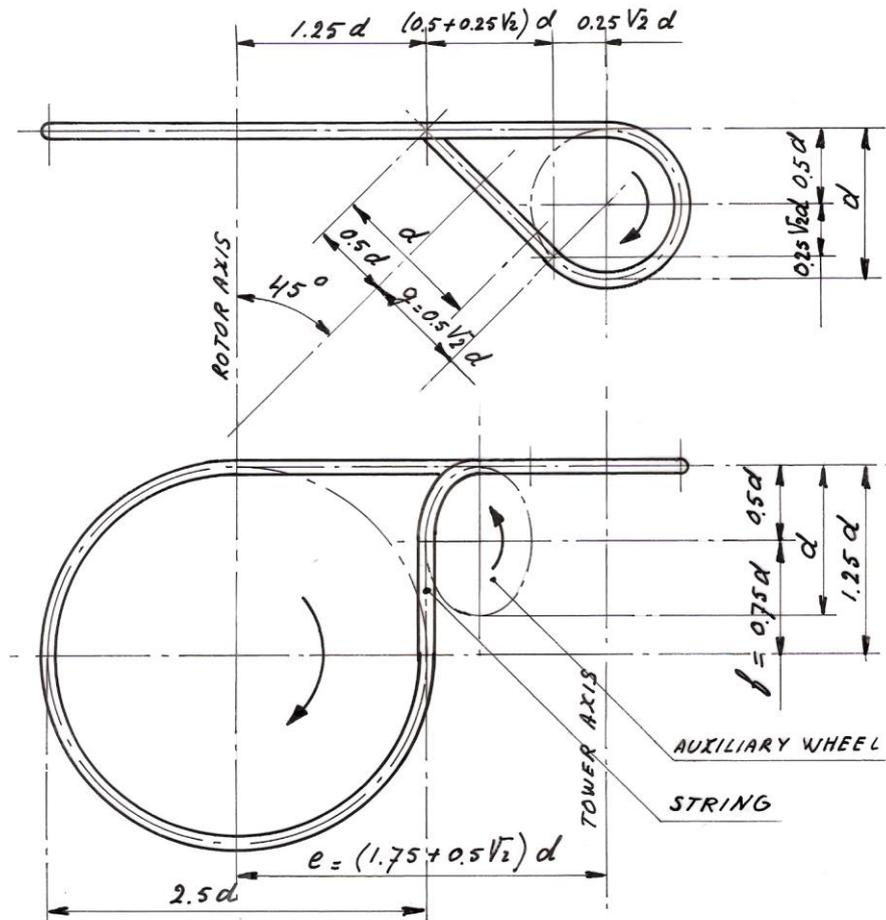
fig. 8 String path and wheels for VIRYA-3.4 transmission with  $i = 2.5$
