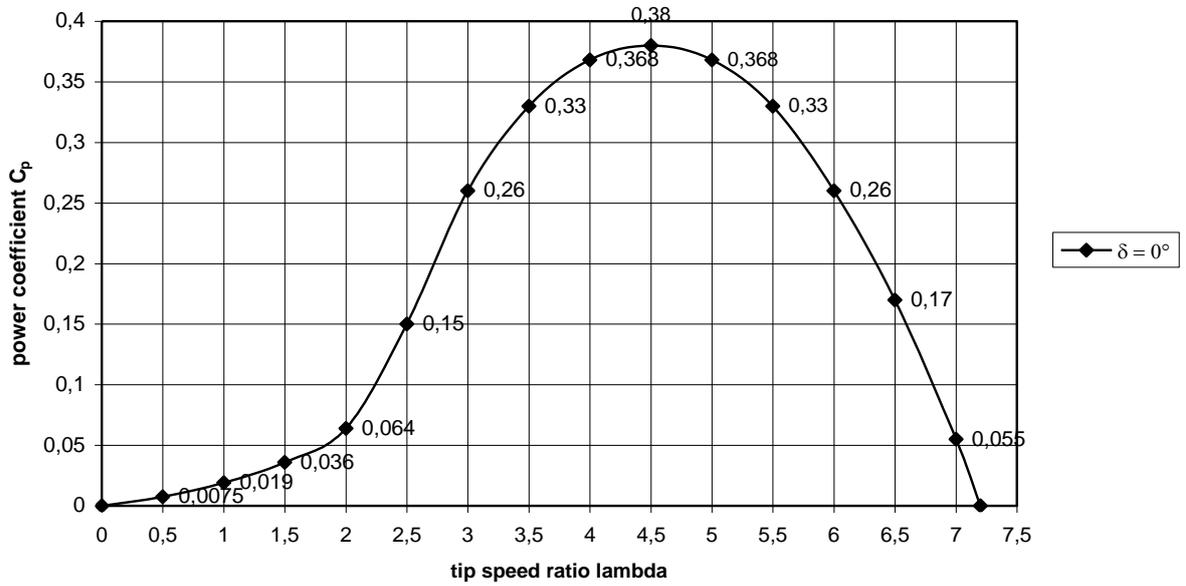
fig. 2 Estimated  $C_p$ - $\lambda$  curve for the VIRYA-3.4 rotor for the wind direction perpendicular to the rotor ( $\delta = 0^\circ$ )
