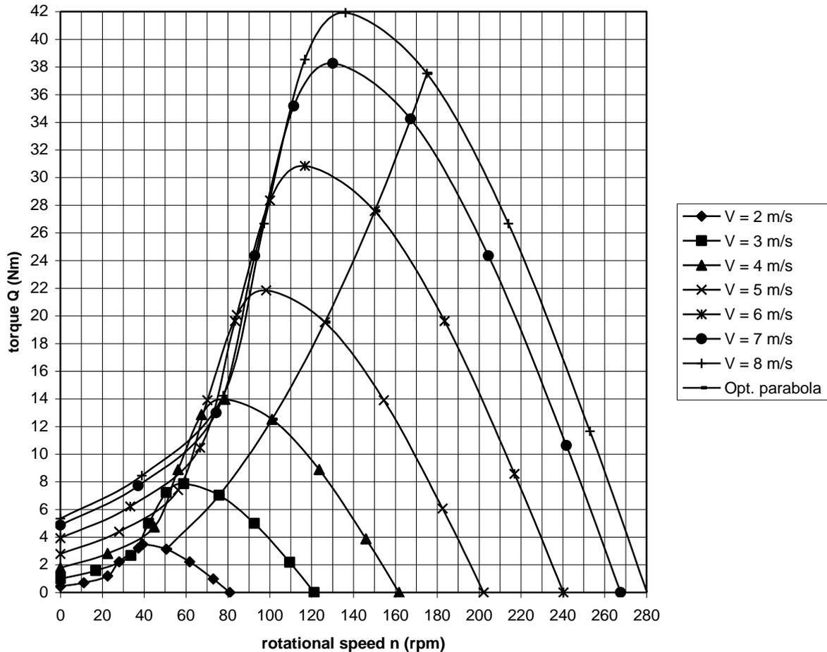
fig. 5 Q-n curves of the VIRYA-3.4 rotor
