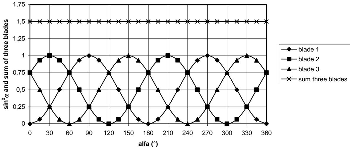
fig. 7 Path of  $\sin^2\alpha$  and the sum of three blades
