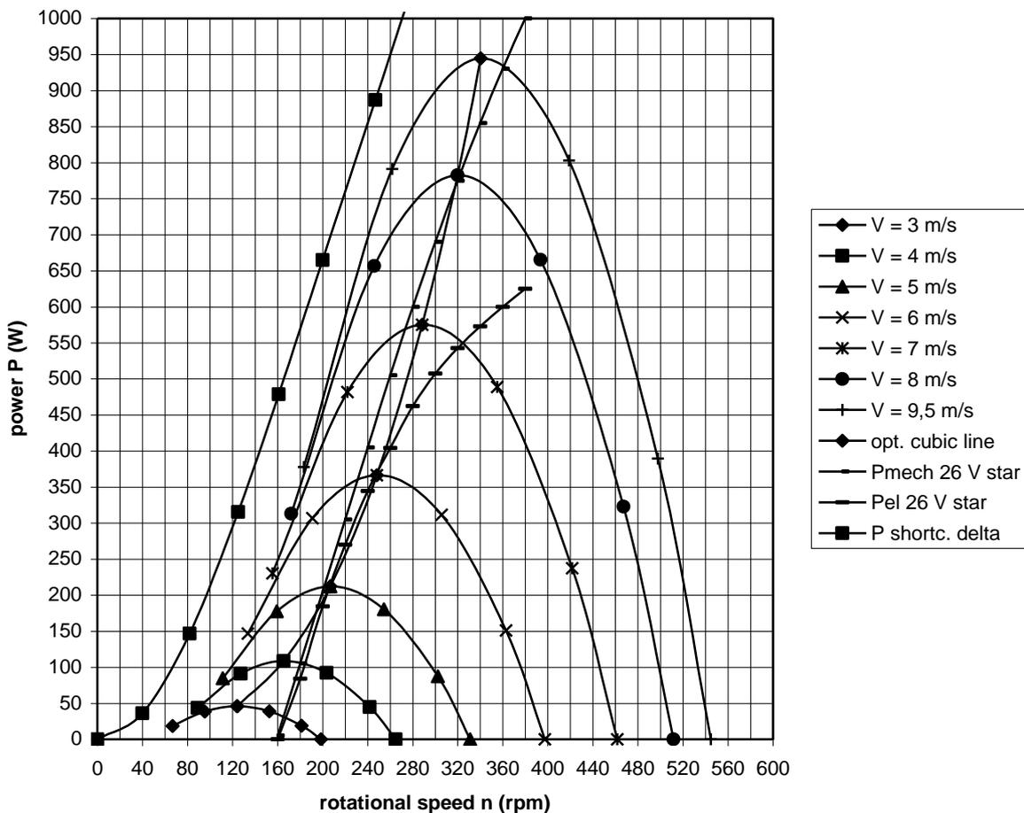
fig. 3  $P$ - $n$  curves of the VIRYA-3B3 rotor for  $V_{\text{rated}} = 9.5$  m/s, optimum cubic line, estimated  $P_{\text{mech}}$ - $n$  and  $P_{\text{el}}$ - $n$  curves of the 12-pole PM-generator for 26 V star, estimated  $P$ - $n$  curve of the generator for short-circuit in delta.
