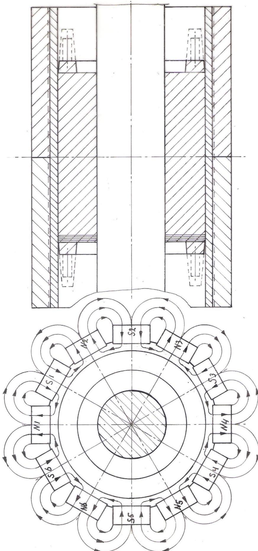
fig. 1 12-pole armature with 24 neodymium magnets size 80 \* 20 \* 10 mm.
