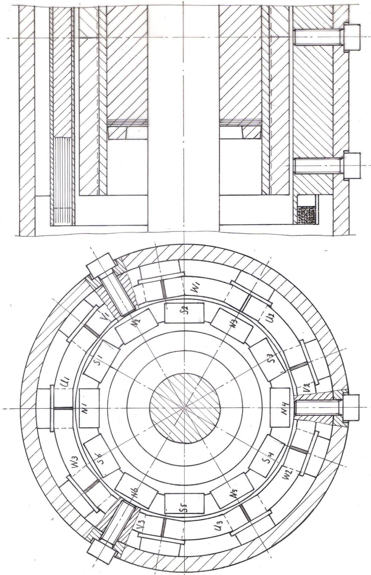
fig. 2 12-pole PM-generator, 3-phase stator with a 1-layer winding with three coils per phase
