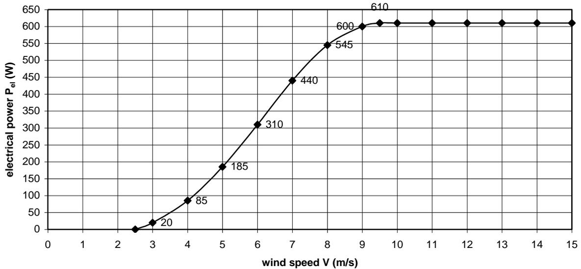
fig. 4 Estimated  $P_{el}$ -V curve VIRYA-3B3 for 24 V battery charging
