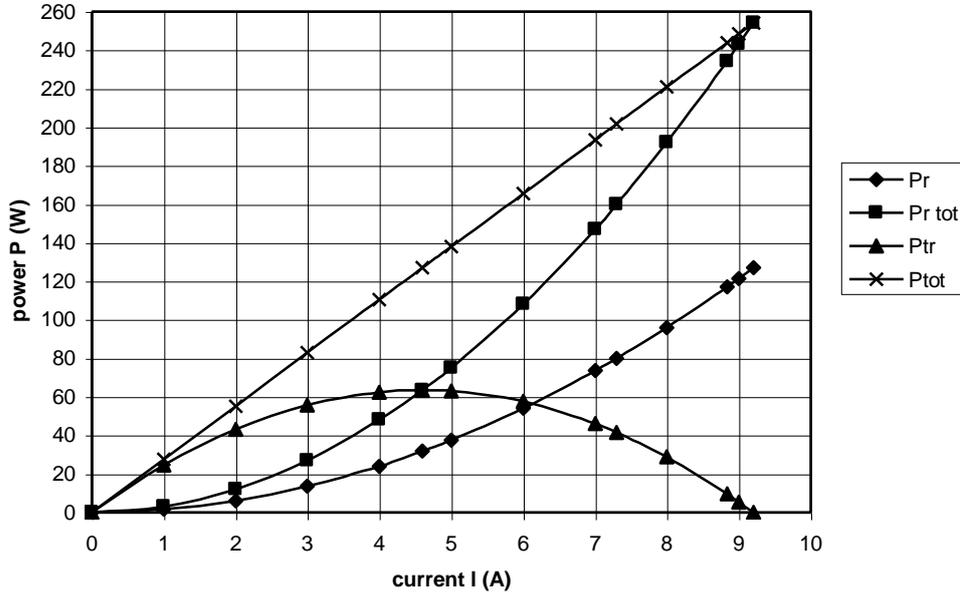
fig. 4 Variation of  $P_r$ ,  $P_{r\ tot}$ ,  $P_{tr}$  and  $P_{tot}$  as a function of  $I$  for  $U_{batt} = 27.6$  V and  $R = 1.5$   $\Omega$
