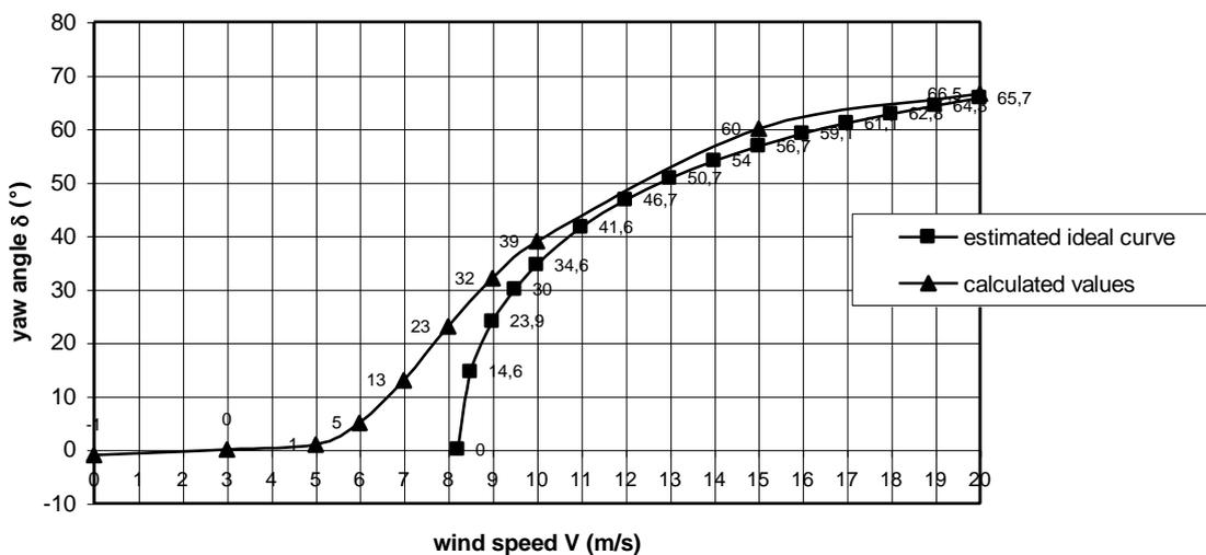
figure 14 The estimated ideal en the calculated  $\delta$ -V curve of the VIRYA-4.2 windmill for  $V < 20$  m/s and with added values for the calculated curve for  $V = 3, 7, 8$  and  $9$  m/s
