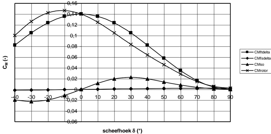
figure 4 Path of  $C_{M_{Ft\delta}}$ ,  $C_{M_{Fs\delta}}$ ,  $C_{M_{s0}}$  and  $C_{M_{rotor}}$  for the VIRYA-4.2 rotor
