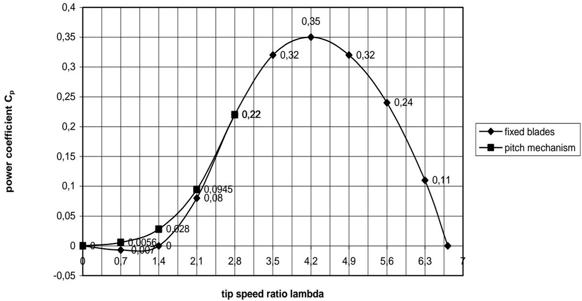
Fig. 3 Estimated  $C_p$ - $\lambda$  curve H-Darrieus rotor with fixed blades and with a pitch mechanism
