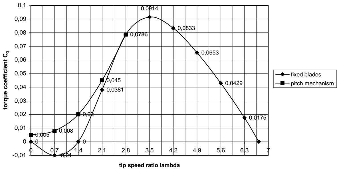
Fig. 4 Estimated  $C_q$ - $\lambda$  curve H-Darrieus rotor with fixed blades and with a pitch mechanism
