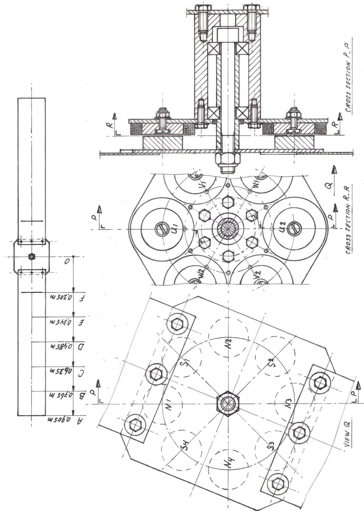
fig. 2 8-pole axial flux permanent magnet generator VIRYA-1.81
