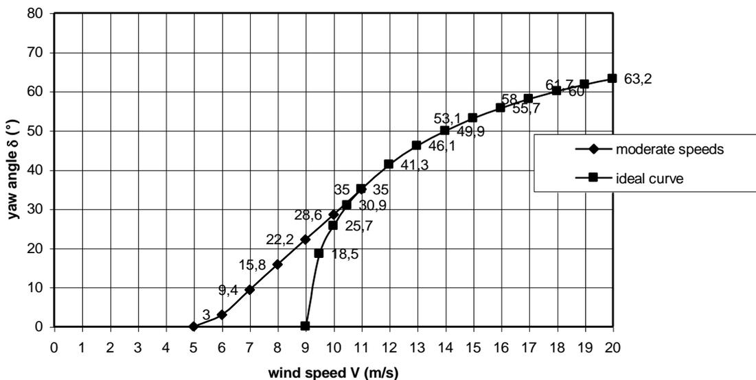
fig. 5 Estimated  $\delta$ -V curve VIRYA-1.81 for a 1 mm stainless steel vane blade
