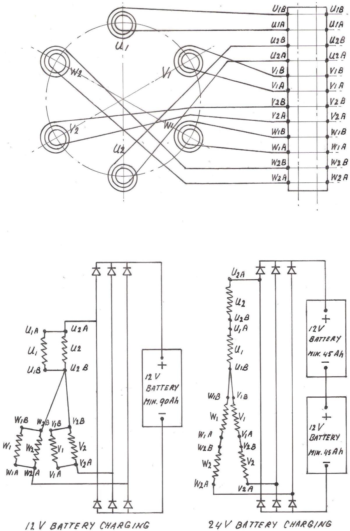
fig. 1 Sketch of the 3-phase winding. Rectification diagram for 12 V and 24 V battery charging
