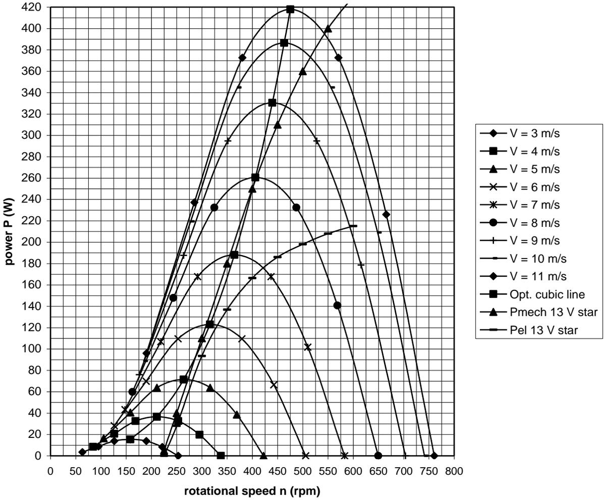
fig. 6 P-n curves of the VIRYA-1.81 rotor and a 1 mm stainless steel vane blade, optimum cubic line, estimated  $P_{mech-n}$  and  $P_{el-n}$  curves for 12 V battery charging for the chosen 12 V / 24 V winding for parallel connection of the two coils of one phase
