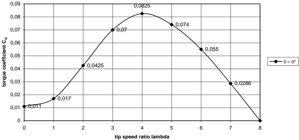
fig. 4 Estimated  $C_q$ - $\lambda$  curve for the VIRYA-1.81 rotor for the wind direction perpendicular to the rotor ( $\delta = 0^\circ$ )
