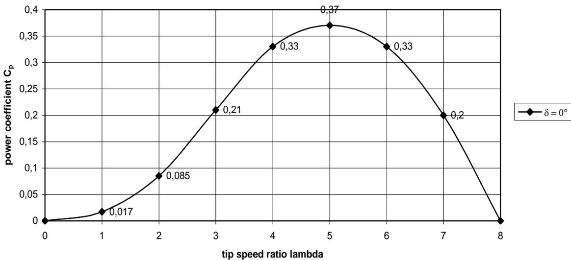
fig. 3 Estimated  $C_p$ - $\lambda$  curve for the VIRYA-1.81 rotor for the wind direction perpendicular to the rotor ( $\delta = 0^\circ$ )
