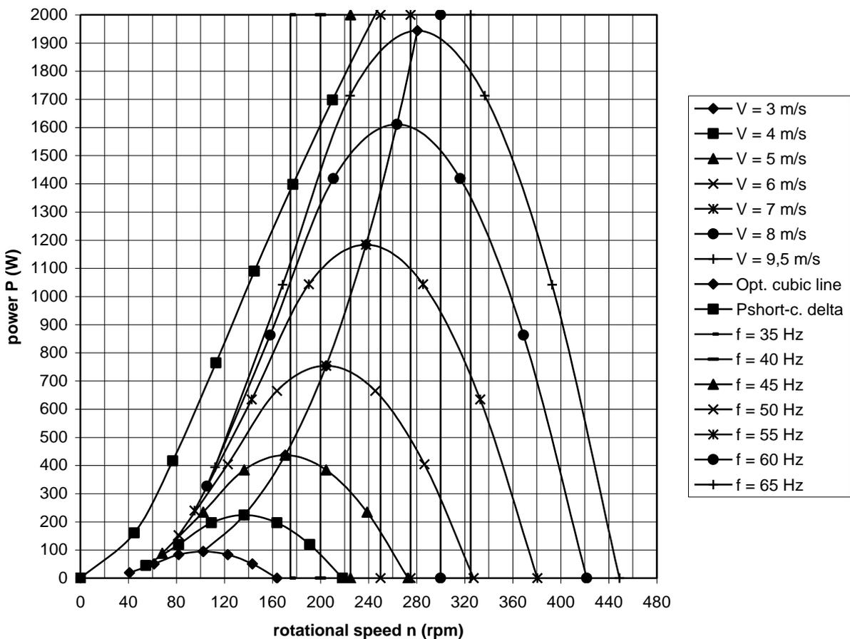
fig. 3 P-n curves alternative VIRYA-4.2 rotor, optimum cubic line, lines for constant frequencies of 35, 40, 45, 50, 55, 60 and 65 Hz.
