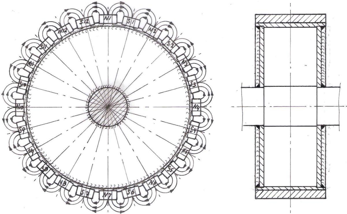
fig. 1 24-pole armature with twenty-four neodymium magnets size 80 \* 20 \* 10 mm.
