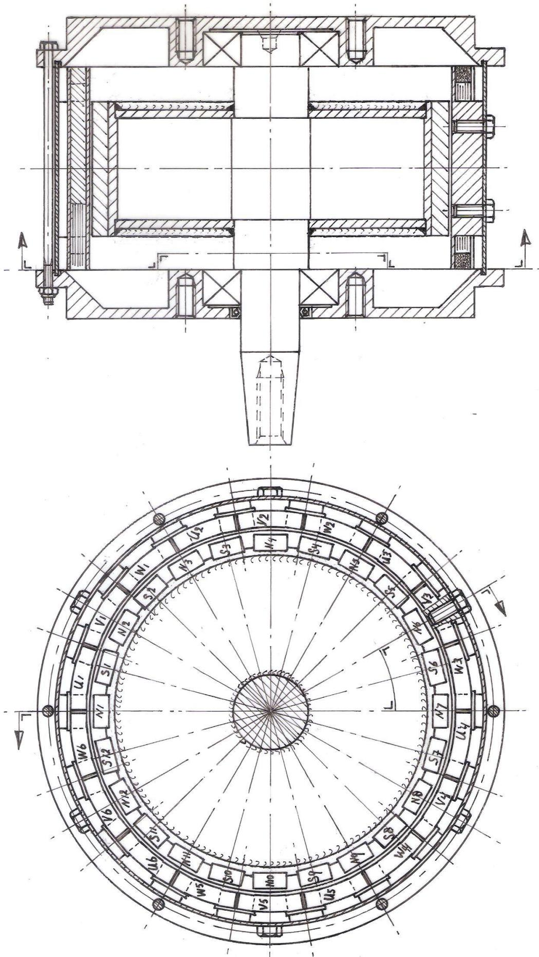
fig. 2 24-pole, 3-phase stator with a 1-layer winding with six coils per phase
