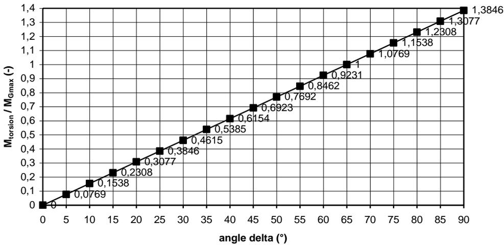
fig. 5  $M_{torsion} / M_{Gmax}$  as a function of  $\delta$
