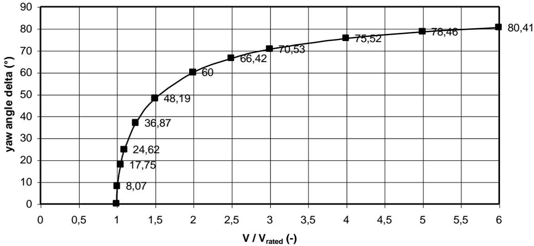
fig. 1 the  $\delta$ - $V/V_{\text{rated}}$  curve for the ideal safety system
