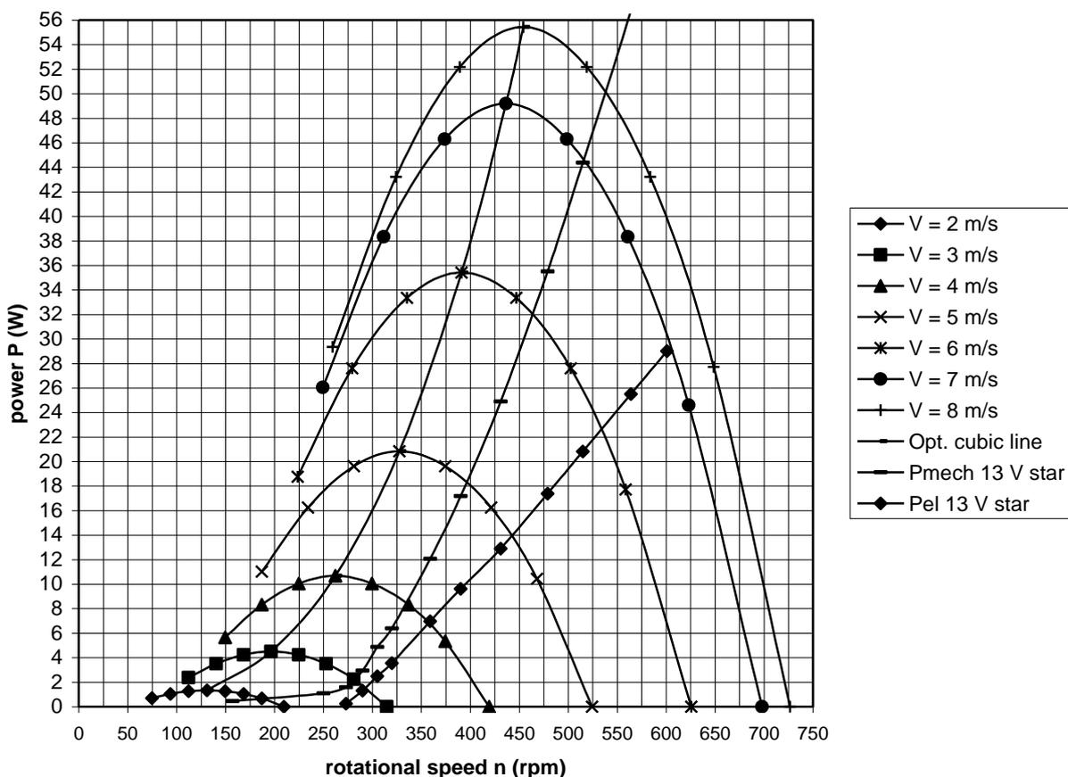
fig. 8 Estimated  $P$ - $n$  curves and optimum cubic line of the VIRYA-1.02 rotor, measured  $P_{\text{mech}}-n$  and  $P_{\text{el}}-n$  curves.
