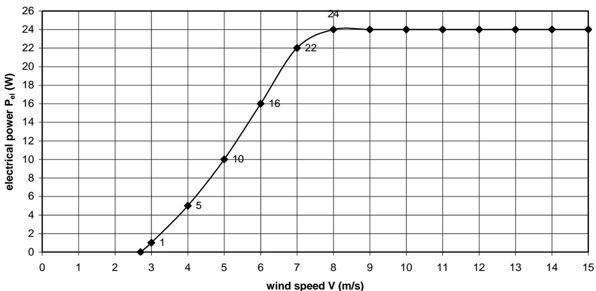
fig. 9  $P_{\text{el}}-V$  curve of the VIRYA-1.02 for measured generator characteristics
