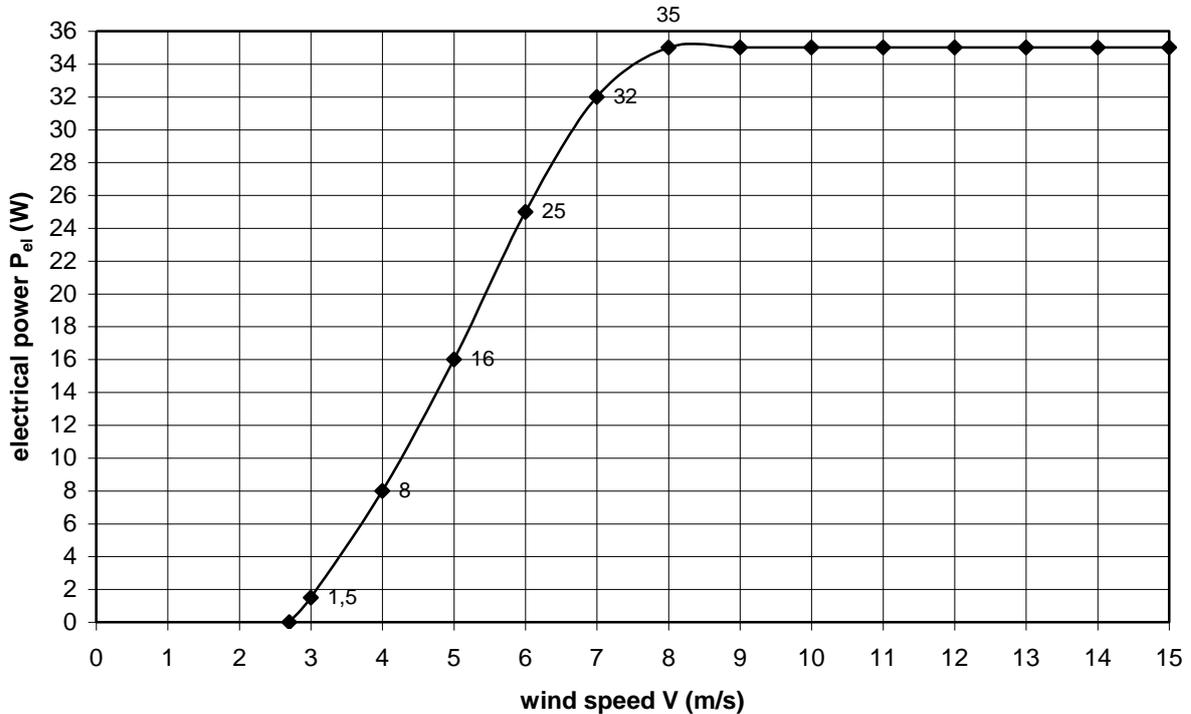
fig. 5 Estimated  $P_{el}$ - $V$  curve of the VIRYA-1.02 windmill for 12 V battery charging
