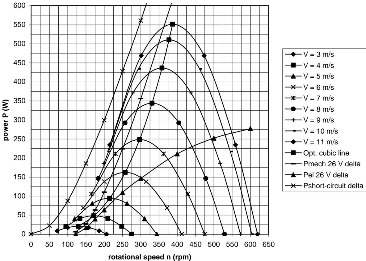
fig. 6 P-n curves and optimum cubic line of the VIRYA-2S rotor, estimated  $P_{mech-n}$  and  $P_{el-n}$  curves for 26 V delta, estimated P-n curve for short-circuit in delta
