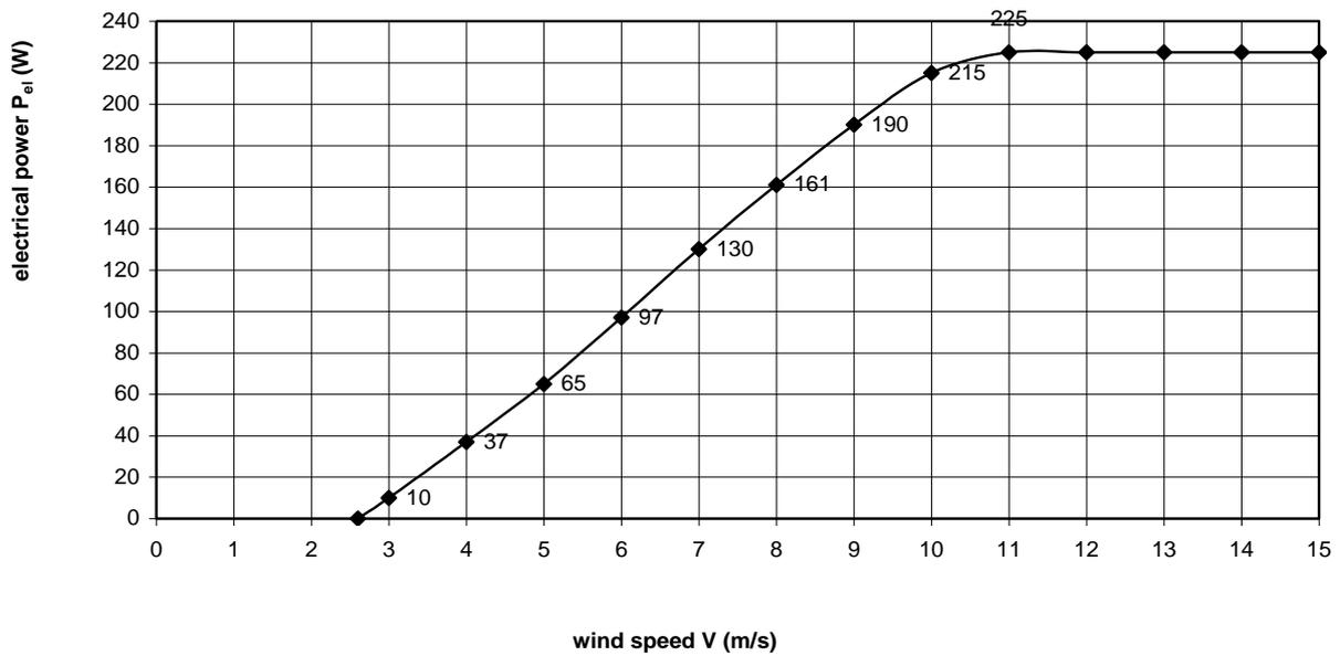
fig. 9  $P_{el}$ - $V$  curve of the VIRYA-2S windmill with  $V_{rated} = 11$  m/s for 52 V star
