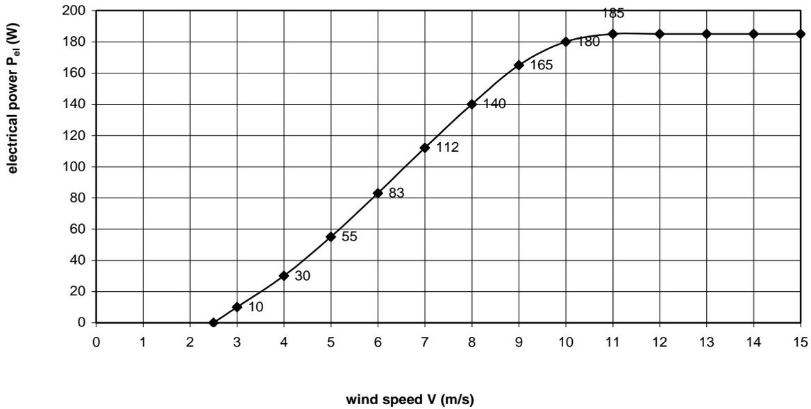
fig. 7  $P_{el}$ - $V$  curve of the VIRYA-2S windmill with  $V_{rated} = 11$  m/s for 26 V delta
