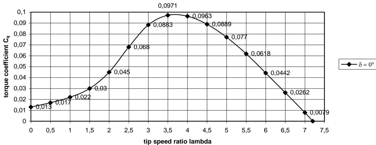
fig. 4 Estimated  $C_q$ - $\lambda$  curve for the VIRYA-2S rotor for the wind direction perpendicular to the rotor ( $\delta = 0^\circ$ )
