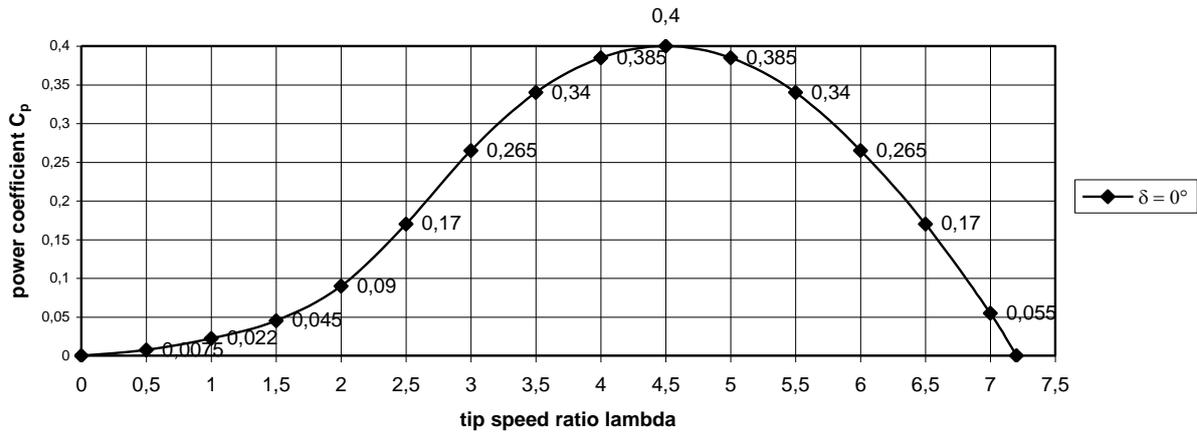
fig. 3 Estimated  $C_p$ - $\lambda$  curve for the VIRYA-2S rotor for the wind direction perpendicular to the rotor ( $\delta = 0^\circ$ )
