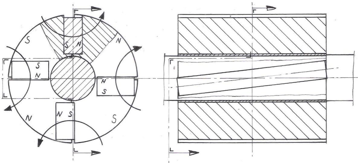
fig. 1 PM-armature of a 4-pole PM-generator frame size 80
