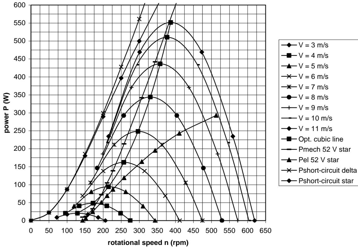
fig. 8 P-n curves and optimum cubic line of the VIRYA-2S rotor, estimated  $P_{\text{mech}}$ -n and  $P_{\text{el}}$ -n curves for 52 V star, estimated P-n curves for short-circuit in delta and in star
