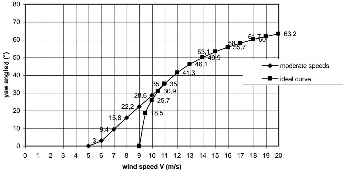
fig. 5 Estimated  $\delta$ -V curve for a 1 mm stainless steel vane blade
