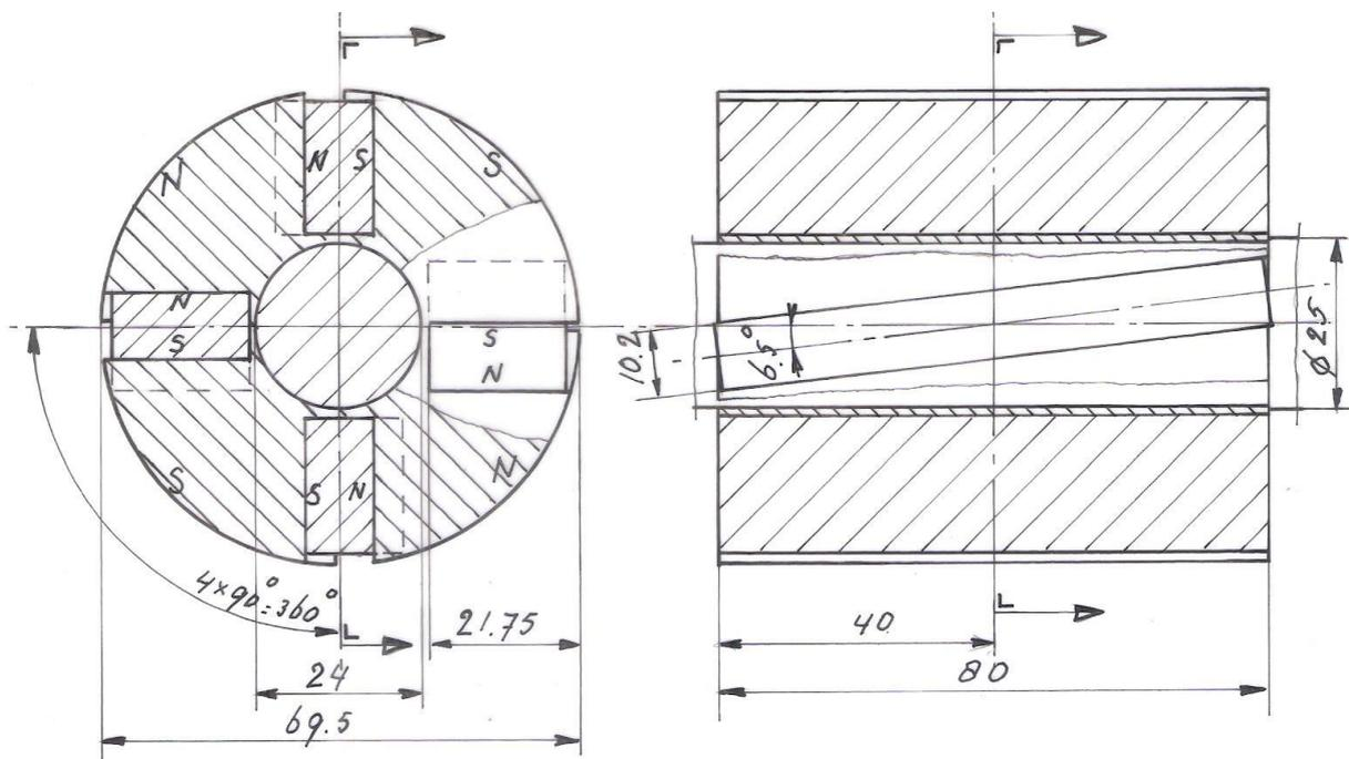
fig. 10 PM-armature of a 4-pole PM-generator frame size 80 with essential measures
