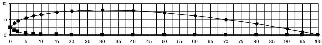
fig. 1 Gö 622 airfoil for c = 100 mm
