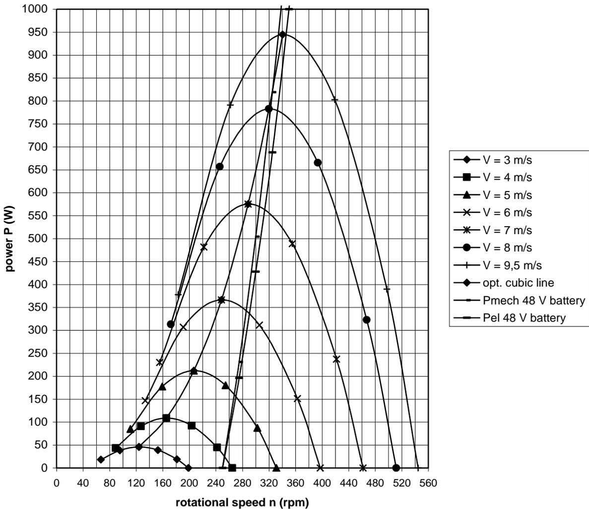
fig. 1 P-n curves of the VIRYA-3B3 rotor for  $V_{rated} = 9.5$  m/s, optimum cubic line, estimated  $P_{mech-n}$  and  $P_{el-n}$  curves of the generator type TGET320-1KW-350R for 48 V battery charging, rectification in star.
