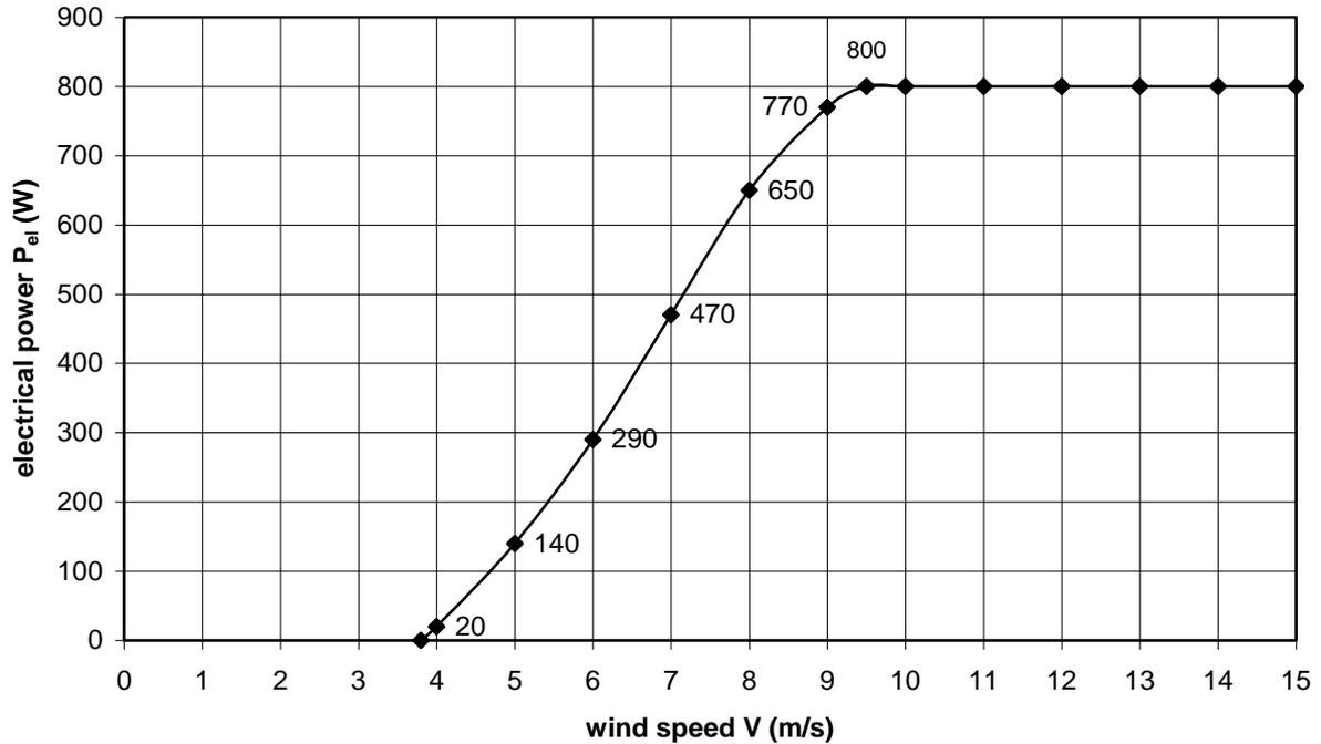
fig. 2 Estimated  $P_{el}$ - $V$  curve of the VIRYA-3B3 windmill with a generator of Hefei Top Grand type TGET320-1KW-350R for 48 V battery charging
