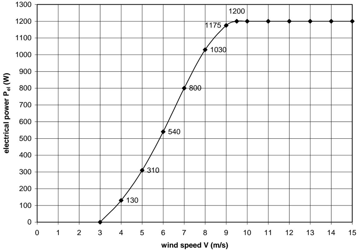
fig. 7  $P_{el}$ - $V$  curve for 52 V star
