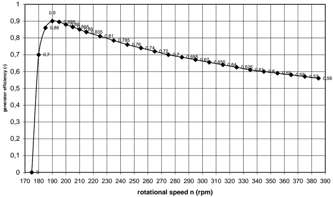
fig. 6 Estimated  $\eta_{\text{gen}}$ - $n$  curve for 52 V star
