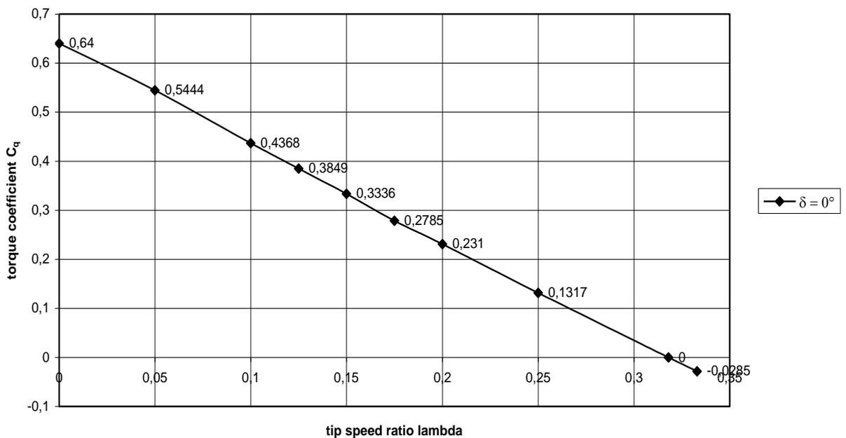
fig. 3 Calculated  $C_q$ - $\lambda$  curve for a drag machine with half hollow spheres
