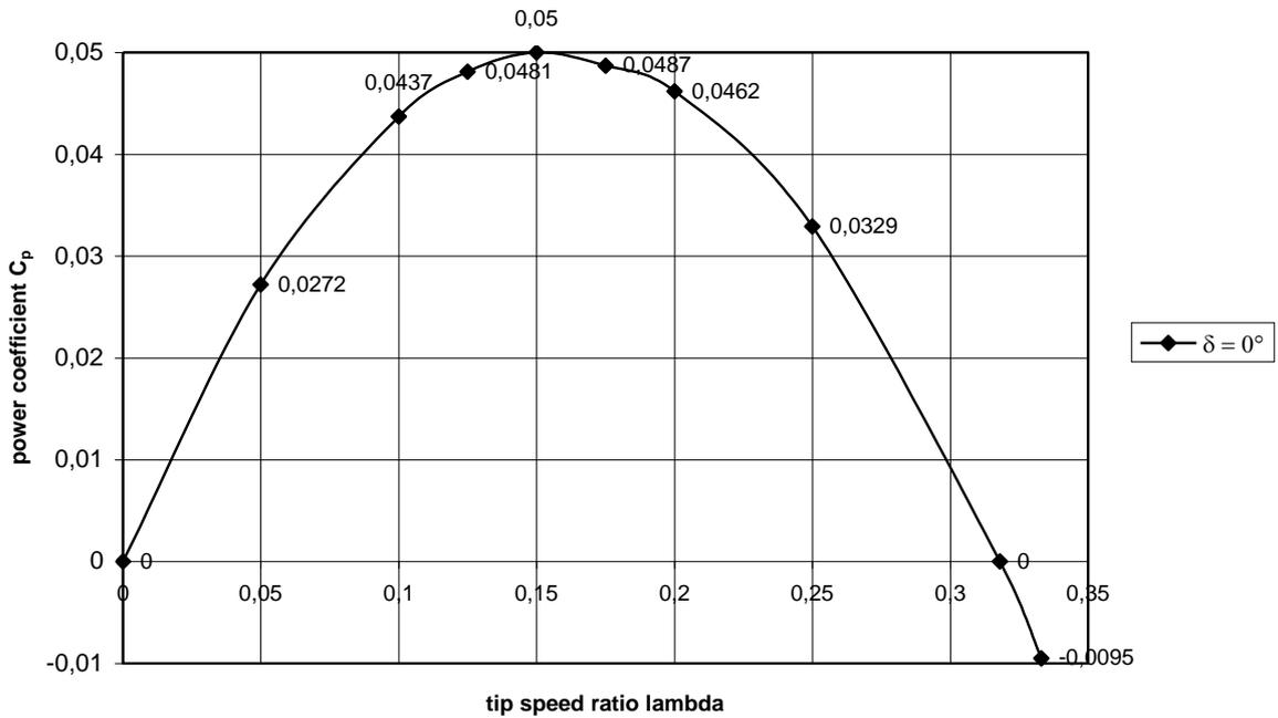
fig. 2 Calculated  $C_p$ - $\lambda$  curve for a drag machine with half hollow spheres
