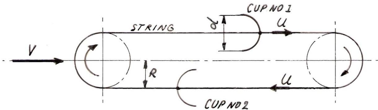
fig. 1 Cup no 1 and cup no 2 mounted on a string parallel to the wind direction
