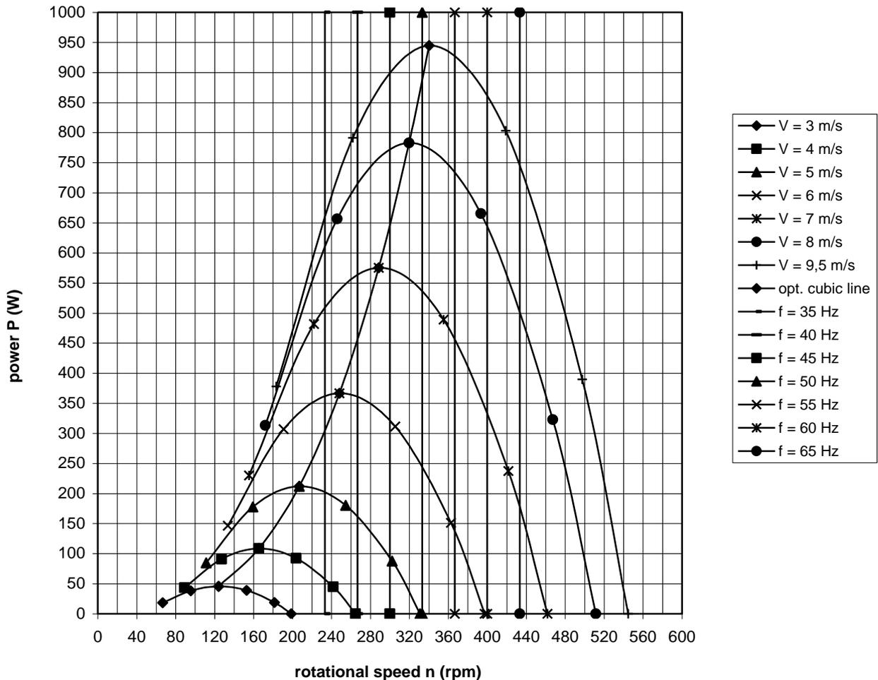
fig. 3 P-n curves of the VIRYA-3B3 rotor for  $V_{\text{rated}} = 9.5$  m/s and optimum cubic line
