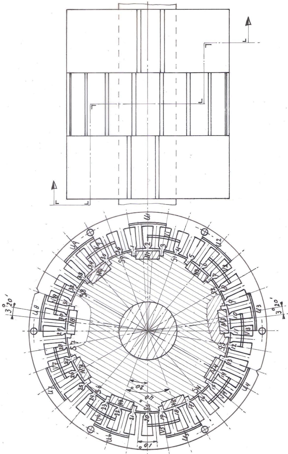
fig. 1 18-pole generator with a 2-layer, 2-phase winding
