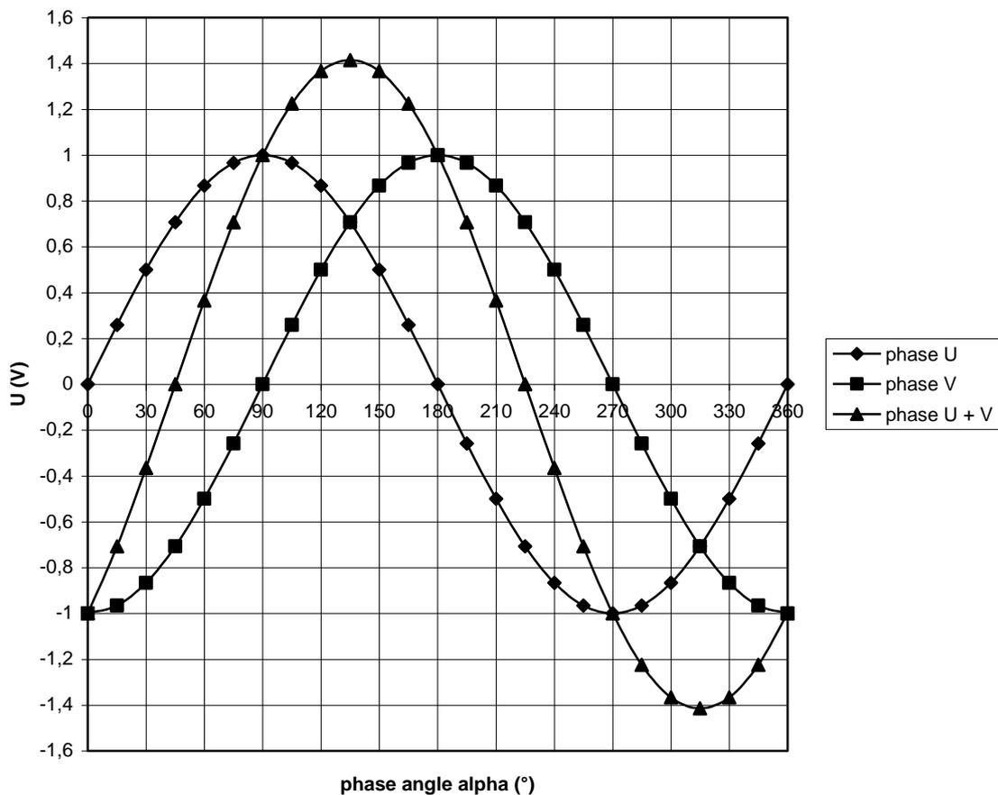
fig. 2 Voltage fluctuation according to formulas 2 – 4 for  $U_{\max} = 1 \text{ V}$ .
