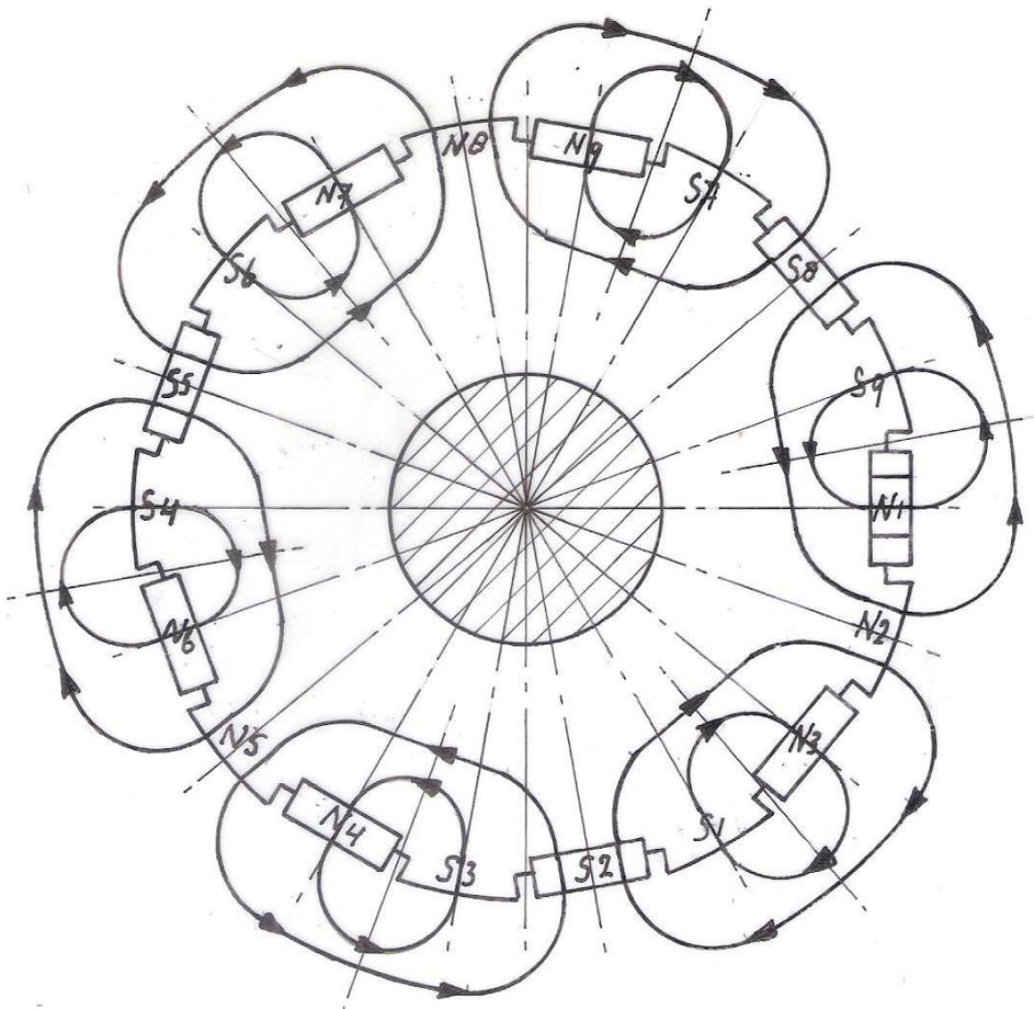
fig. 4 Alternative 6-pole armature combined with the original 6-pole winding
