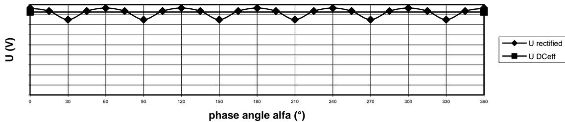
Figure 1 Variation of a 3-phase alternating voltage rectified in star
