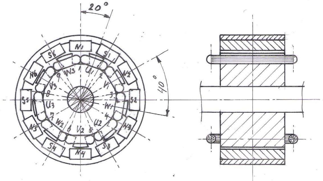
Figure 2 Armature and stator of a 12-pole, 3-phase hub dynamo
