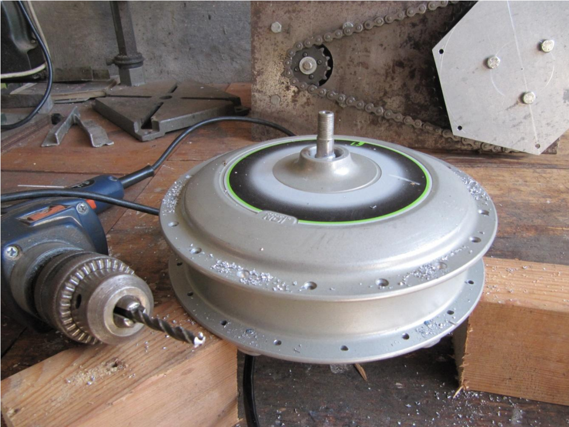
fig. 2 Drilling of six 5 mm holes
