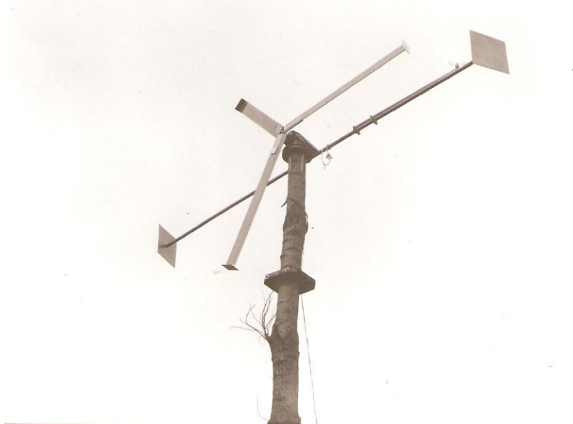
fig. 11 DRIEKA-4 windmill with double vane and tree tower designed in about 1985
