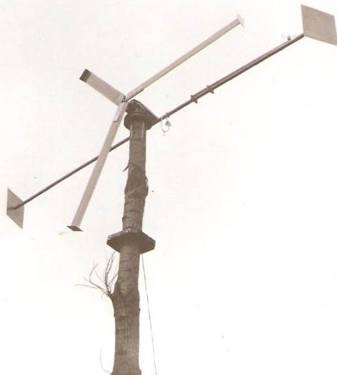
fig. 10 The DRIEKA-4 windmill with double vane and tree tower designed in about 1985
